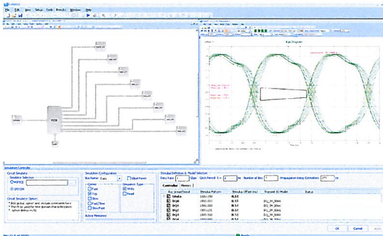
Image #2: SystemSI – Parallel Bus Analysis. Design Topology is synthesized by a wizard to model the complete die-to-die path of high-speed signals together with the PDS.
